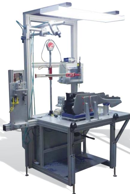
*Operator assisted assembly of an automobile center console. Side panels are pressed into place. Each step and each component is verified by the vision system.*
