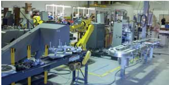
These large robots retrieve parts from the conveyor, then load for debur and sand blast operations. Part is the mixer housing for Kitchenaid.
