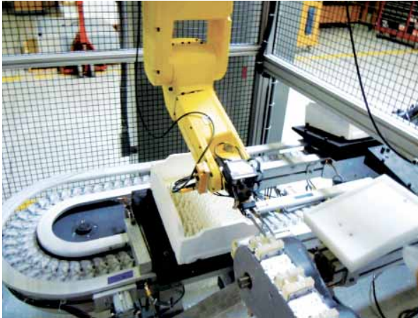
Robot inspect each spark plug insulator and then loads into sagers (containers).
