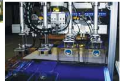
Vision guided Robot works on a conveyor line to pick and place laboratory mice cages. GO2 Technologies also designed the end of arm tooling (GO2 End of Arm Tech ® ) that does the delicate work of picking up the cages.
