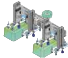
Vision guided Robot works on a conveyor line to pick and place laboratory mice cages. GO2 Technologies also designed the end of arm tooling (GO2 End of Arm Tech ® ) that does the delicate work of picking up the cages.
